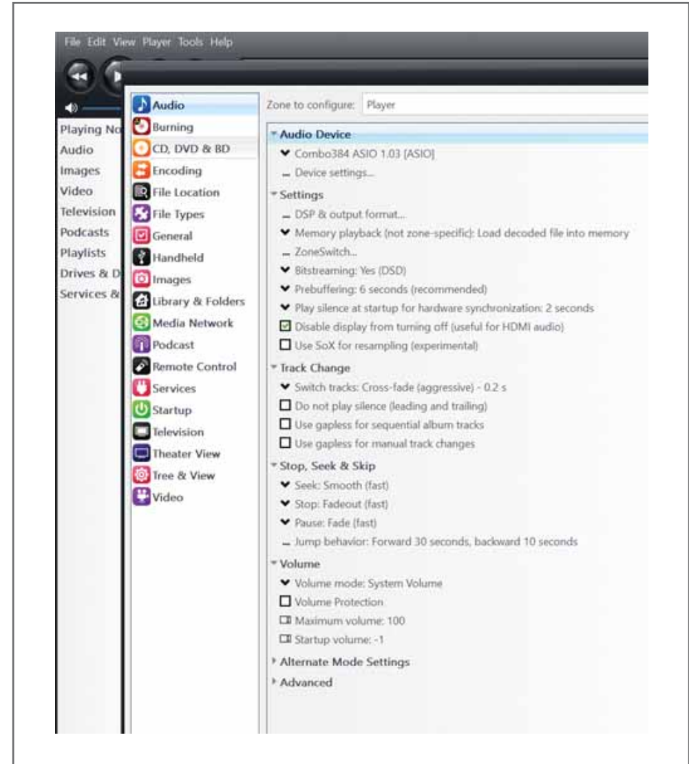
Fig. 8 JRiver MC 22 settings – Windows: When playing DSD files, “Bitstreaming” should be set to “Yes(DSD)”
